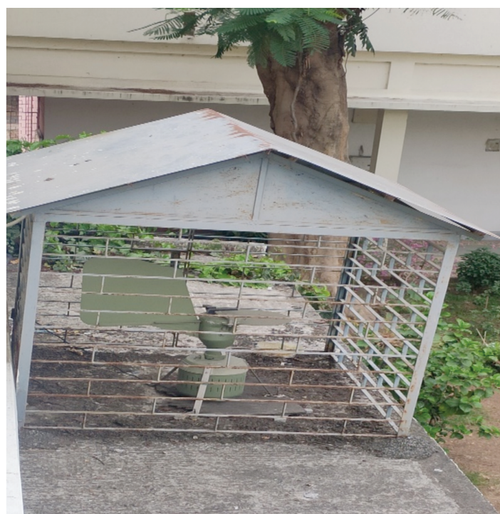
Fig. 3.2: Burkard seven day volumetric sampler placed in the Department of Botany, Visva-Bharati
